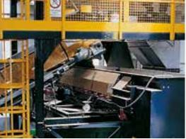
A second magnet is set up before the station of the roll-off containers and separates further metals from the undersize fraction.
