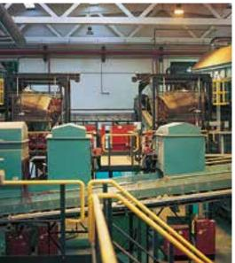
Once the metals have been separated, the mid-size fraction is added back to the large-size fraction coming from the rotary screen. These two fractions together constitute the material that is treated to produce fuel.
