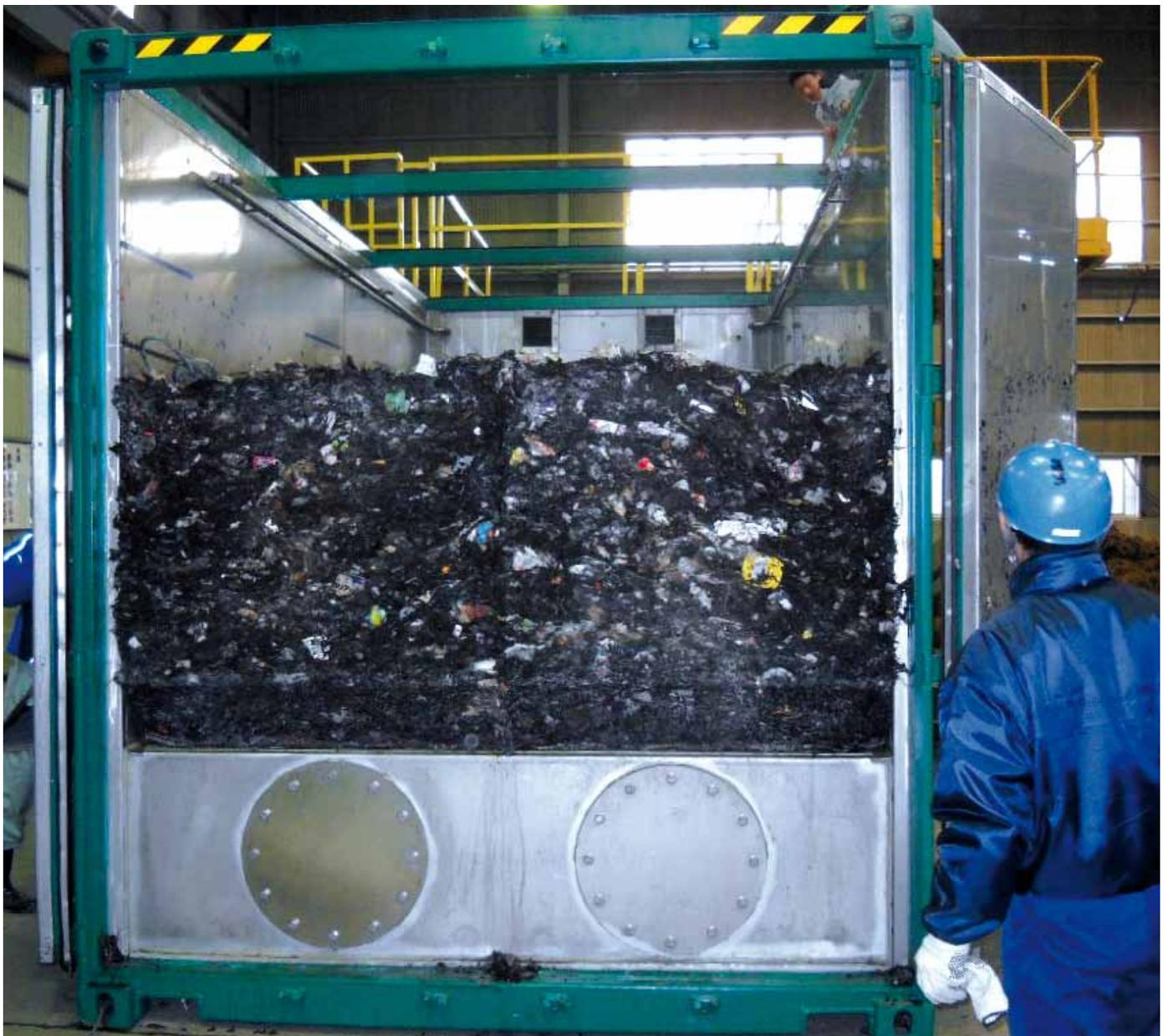
Thanks to a detailed study of the space arrangement, all equipment is installed in a commercial size container (40 foot long), which is divided into three specialized sections:
