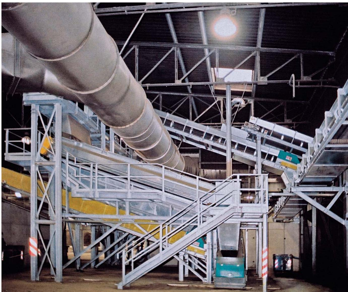
The production of quality compost to be used in agriculture requires the refining of the composted material by means of a screening process. The purpose of this process is to produce a material with a fine particle size, substantially free of contaminants such as plastics, textiles, etc.
