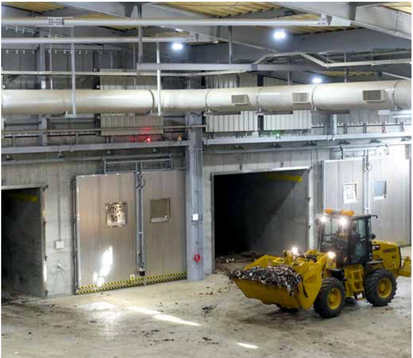
After a mechanical pre-treatment process, the material to be converted to RDF is loaded by a wheel loader into six bio-drying tunnels.
