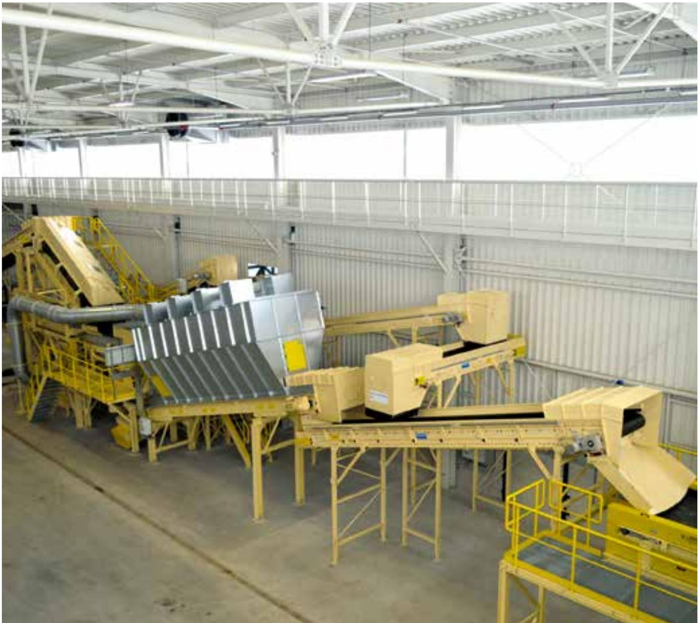
Pre-shredding of mixed MSW (Municipal Solid Waste) is required to facilitate the following sorting process. A slow-speed primary shredder is used to open and empty the bags containing the waste and, at the same time, reduce the particle size of the various waste components.
