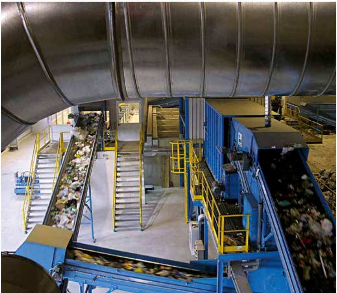
The recyclable waste sorting plant includes various lines which, depending on the type of waste processed, can be combined with great flexibility. Paper and cardboard, mixed with plastic containers and plastic bags, are automatically sieved before being subject to manual sorting (positive or negative), while steel and aluminium cans are automatically sorted from non-metallic waste.
