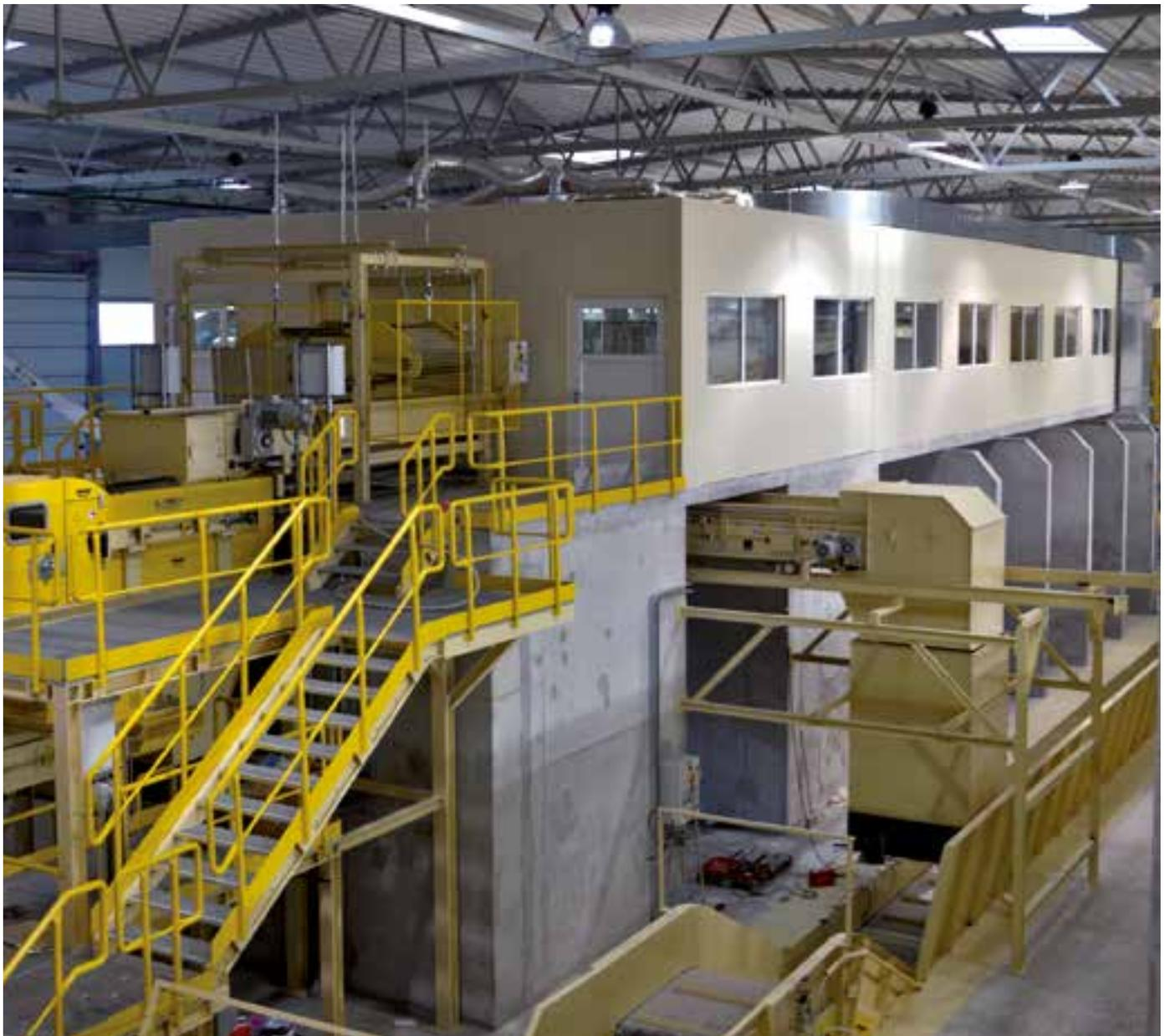
The feeding bag opener is loaded by the mobile equipment and provides for the opening and emptying of the waste containing bags.
