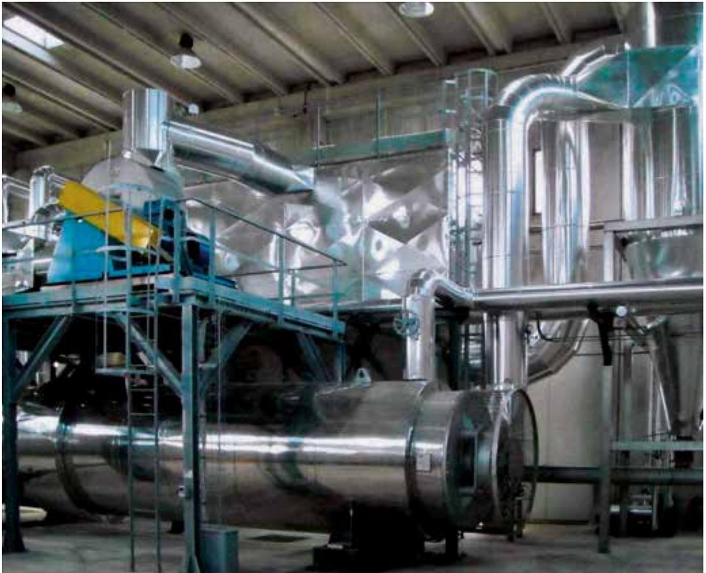
The sludge to be processed is unloaded by the transport vehicles directly in a storage hopper where it is extracted and then conveyed to the drying line. The drier consists of a cylindrical double wall construction, which is heated by diathermic oil. An internal rotor projects the sludge towards the heated wall.
