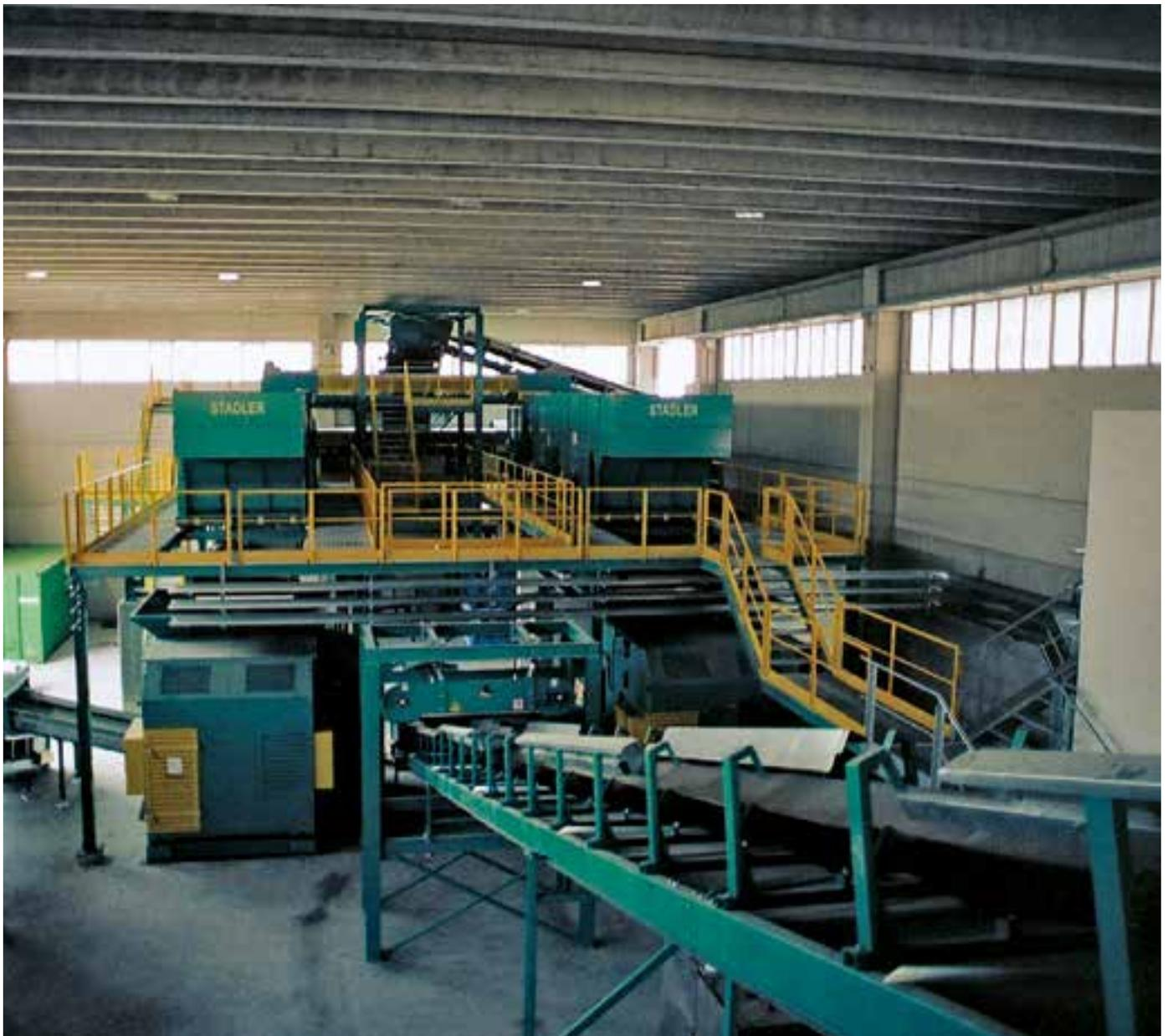
This system treats special non-hazardous waste, as well as the light fraction deriving from the sorting of municipal solid waste.
