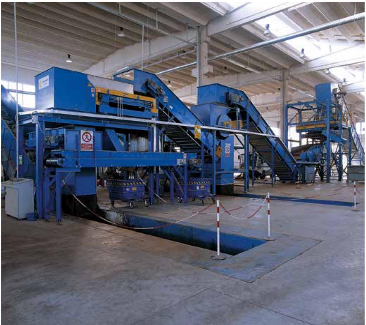
The plant is designed to sort recyclable materials from source-separated municipal waste.
