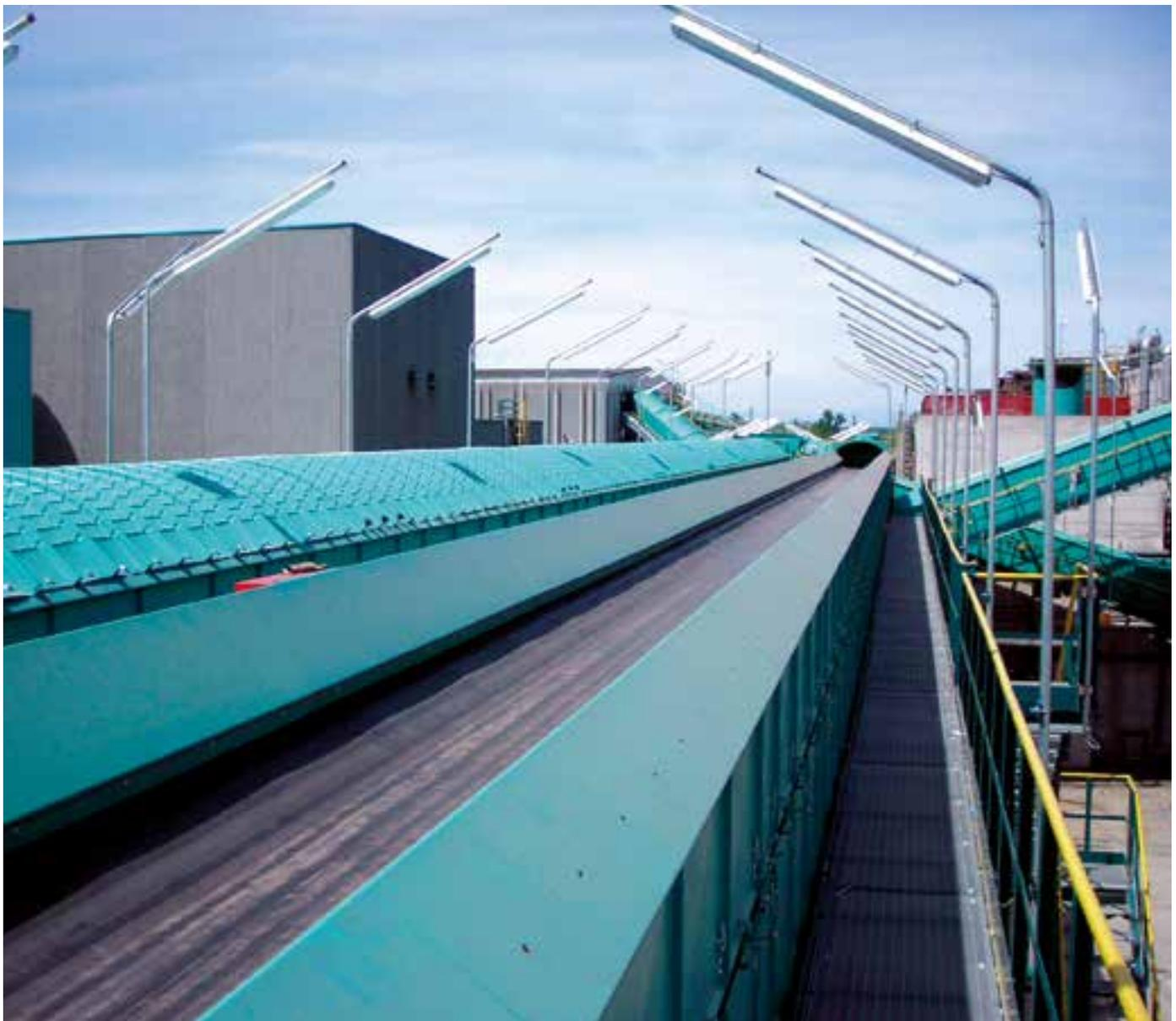
The fourth waste sorting line is designed for the treatment of industrial and commercial waste, consisting mainly of packaging materials and similar wastes. The bulky nature of the processed waste has required the use of a special double rotor, slow-speed primary shredder, which is able to reduce the particle size of the waste to facilitate the sorting operations that follow.
