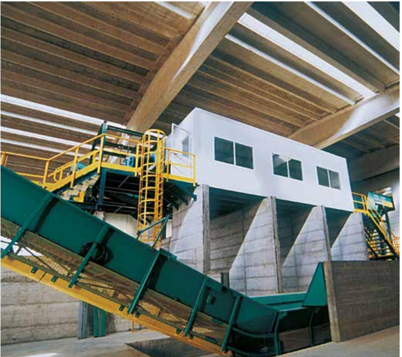
This material recovery facility is de-signed to process commingled recyclable materials deriving from source separation of municipal waste.
