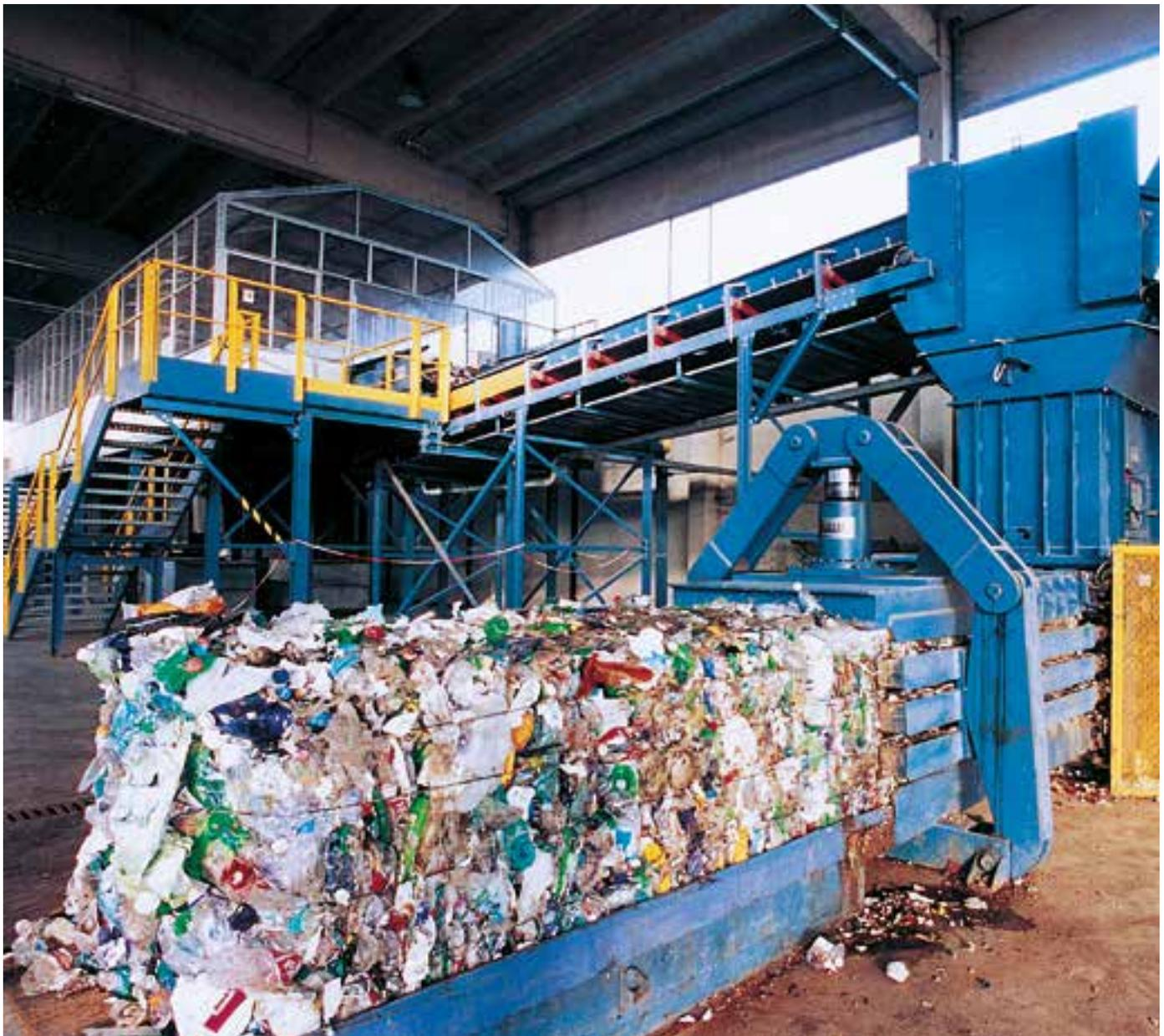
This sorting and baling plant is designed for the treatment of large size recyclable waste, especially pack-aging materials from commercial and industrial facilities.
