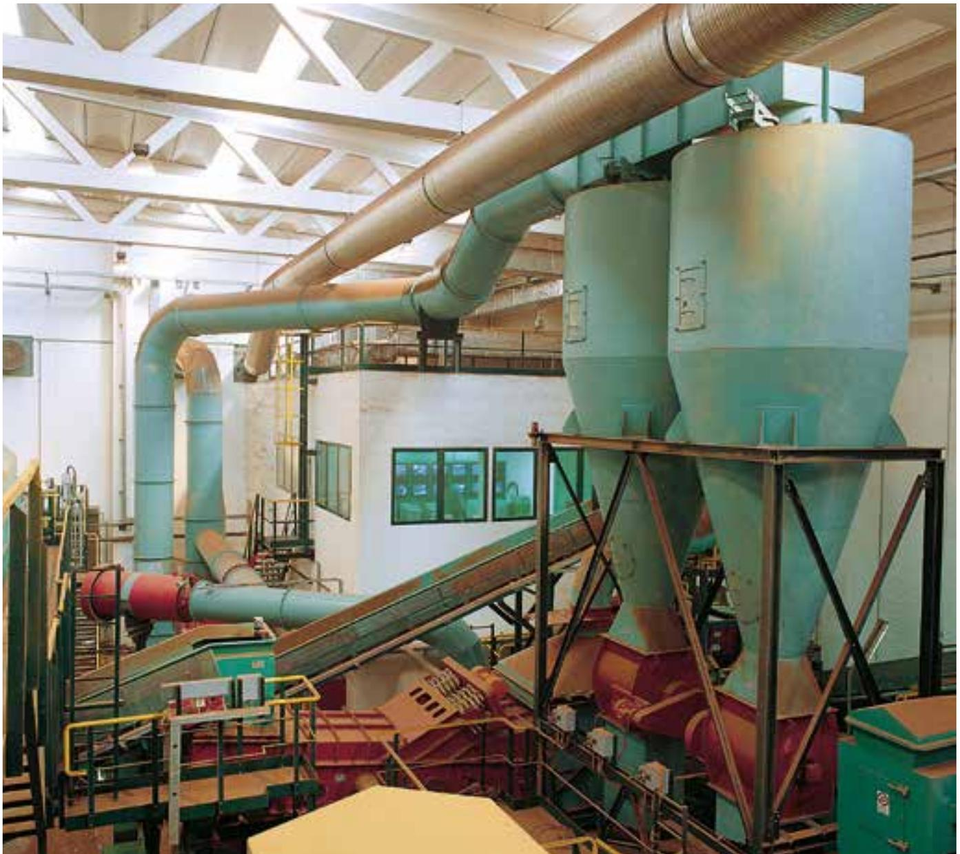
A compost refining system is used to separate inert and combustible material from the stabilized organic fraction produced in the composting building.
