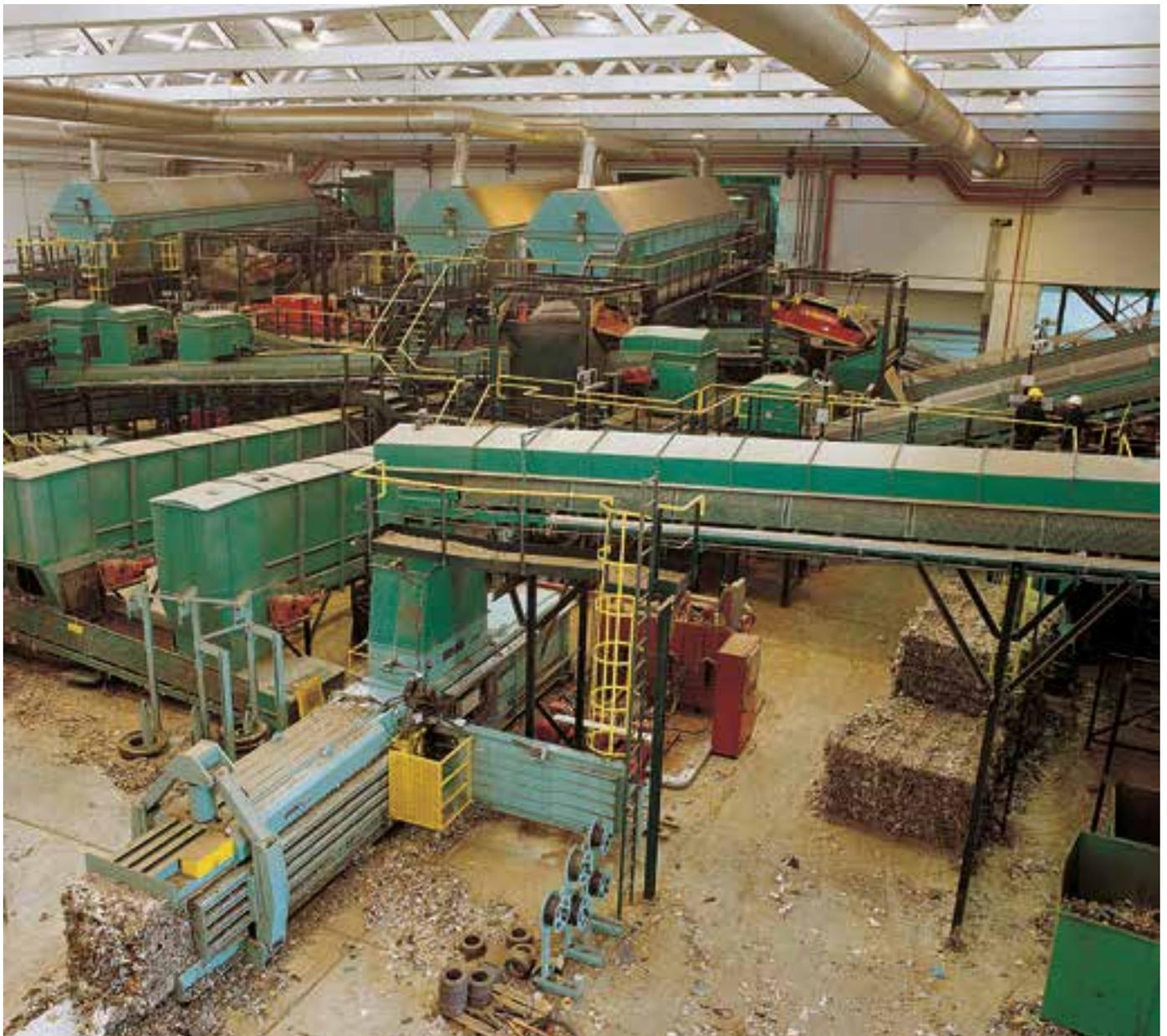
Ecomaster supplied a turnkey system for producing RDF (refuse derived fuel) and stabilizing the organic fraction of municipal waste, which is part of the Lomellina Energia waste-to-energy project. This facility, generating electric power from municipal solid waste, was built by Foster Wheeler Italiana for Lomellina Energia, owner and operator of the project.
