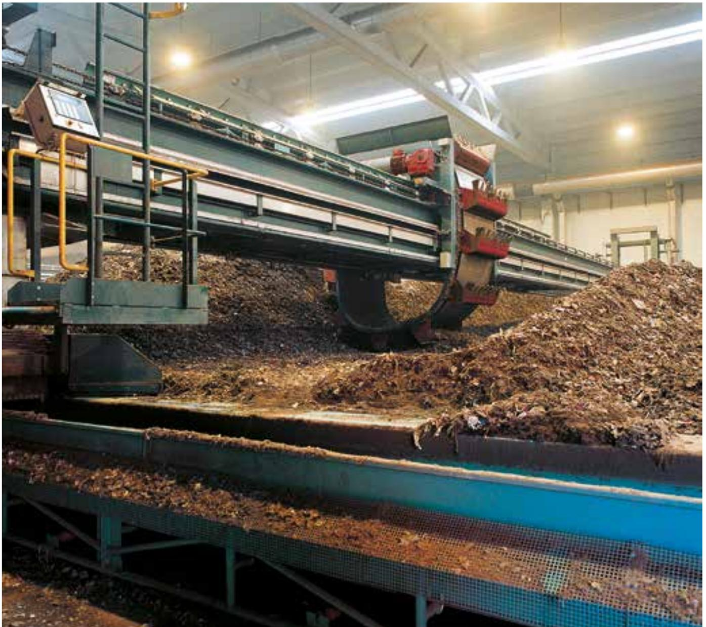
The small-sized material produced by the screens in the sorting area of the plant is collected by conveyor belts and transferred to the adjacent building to go through a biological stabilization process. Before entering the building, the material is processed by a magnet, which separates small-sized ferrous materials.
